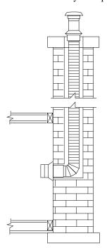
Figure 26 - Straight Installation into Masonry Chimney
